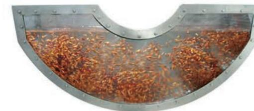
Product passes through standard blancher designs in a deep, dense mass, which can result in overcooking product towards the outside, without reaching the center. Lyco's patented agitation gently rotates product to ensure a thorough, even cook.
