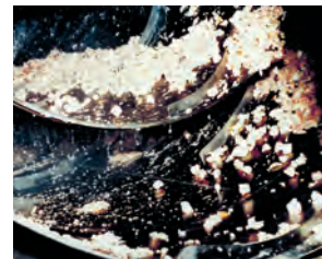
This photo of diced potatoes shows how the inner .080 in screen retains larger particles so the .020 in outer screen can operate more efficiently with less loading.
