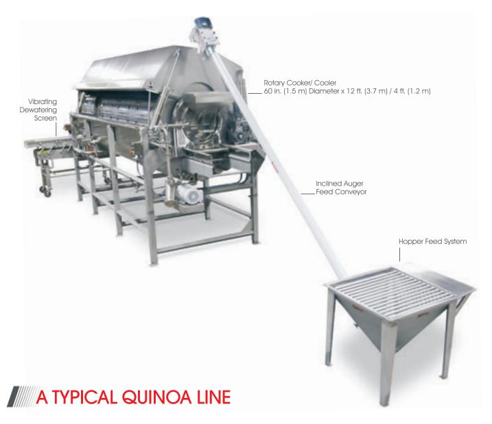
Grain is typically fed into the machine through an inclined auger feed conveyor. In the machine, cylinders consist of augers that are covered by perforated skin sheets. Cylinders are half submerged in a partitioned tank. The cook zone is heated with live steam and the cold zone is cooled with cold or chilled water. Each zone is driven separately for maximum control and efficiency all in a smaller footprint.
