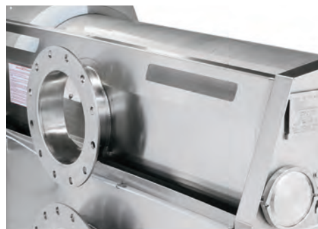
HEADBOX WITH OVER-FLOW FOR PROTECTION
