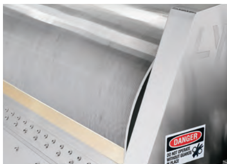
WEDGEWIRE SCREEN CONSTRUCTION IS LESS APT TO PLUG
